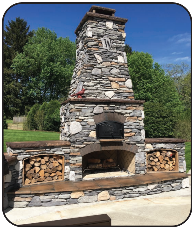
70/30 mix of Prestige Monterey ledgestone and Bluegrass fieldstone with Casa di Sassi Terra chiseled capstones and Brown brick soldier courses
